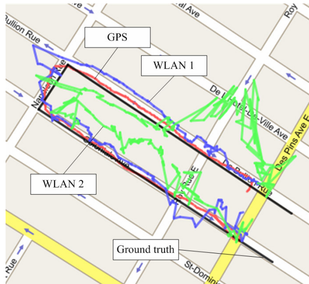
Figure 2. Location estimates obtained by GPS, and WLAN. WLAN 1 refers to the algorithm using a radio map based on GPS, while WLAN 2 refers to the same algorithm based on a radio map based on our automatic indoor mapping algorithm.
